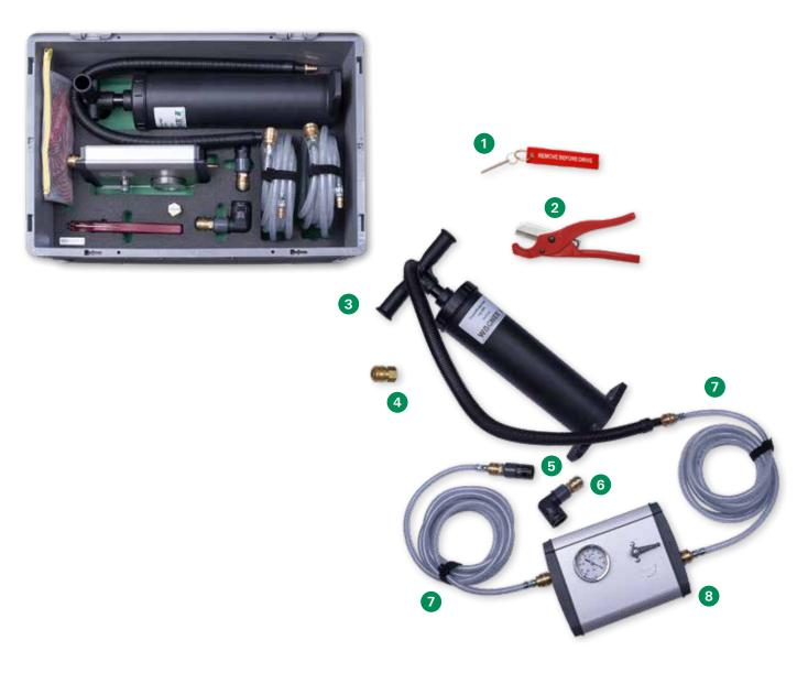
The leakage test set is used to check an air sampling hose system for air sampling smoke detectors for leaks and for professional installation. An energy-independent vacuum measurement allows a quality check to be performed immediately after completing the installation before claddings or similar make access difficult or impossible. The enclosed tools enable immediate repair of damaged areas. The
